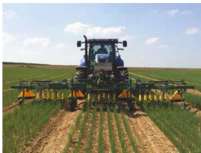
Figure 17 A Micron varidome shielded sprayer in use in salad onions in the UK
