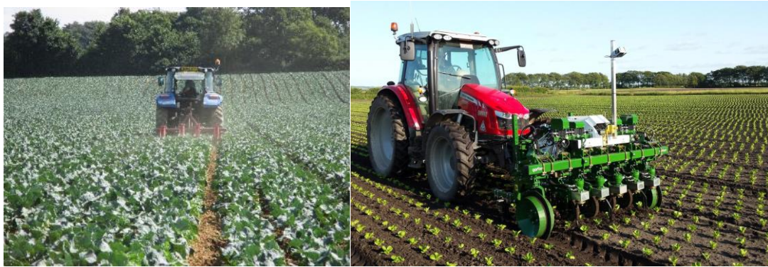
Figure 14 Left. Inter-row hoe guided by GPS. Right. Garford In-row weeder
