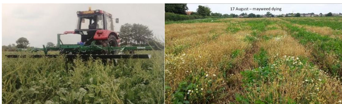
Figure 18 Garford weed wiper in sugar beet (Left), and mayweed dying in a parsnip crop after ‘weed wiping’ with glyphosate (right).
