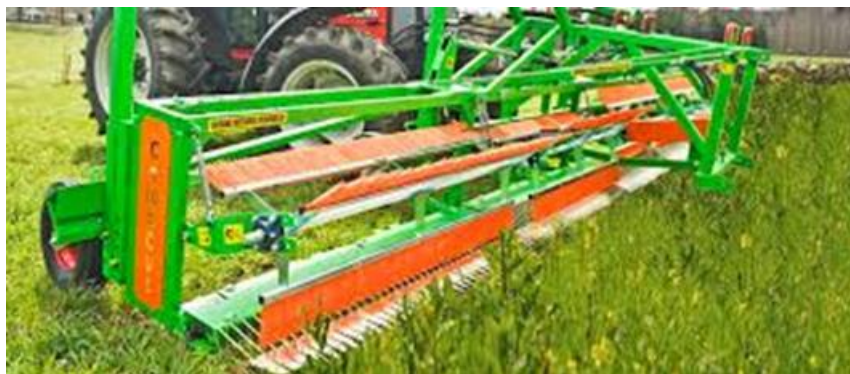
Figure 8: CombCut weed cutter
